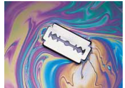
Figure 37.17 A thin film of oil floating on water displays interference, as shown by the pattern of colors produced when white light is incident on the film. Variations in film thickness produce the interesting color pattern. The razor blade gives one an idea of the size of the colored bands.
